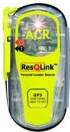
**Personal Locator Beacons (PLBs)** are hand held emergency devices that use satellite technology to **locate individuals lost, injured, or stranded** in the wilderness. When activated, **PLBs send a distress signal** received by SARSAT (Search and Rescue Satellite Aided Tracking) satellites. The distress information including **location coordinates** is then passed to the appropriate **search and rescue organization, all in a matter of minutes.** Search and
